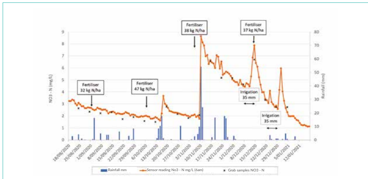
Figure 1: Changes in sump nitrate-nitrogen concentration over the cropping period. Both sensor and grab sample nitrate-nitrogen concentrations are shown along with rainfall, irrigation and fertiliser applications
