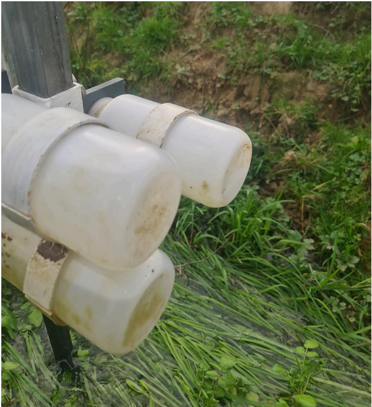
Figure 16: Sampler set to avoid background inflow not associated with a rainfall event.
