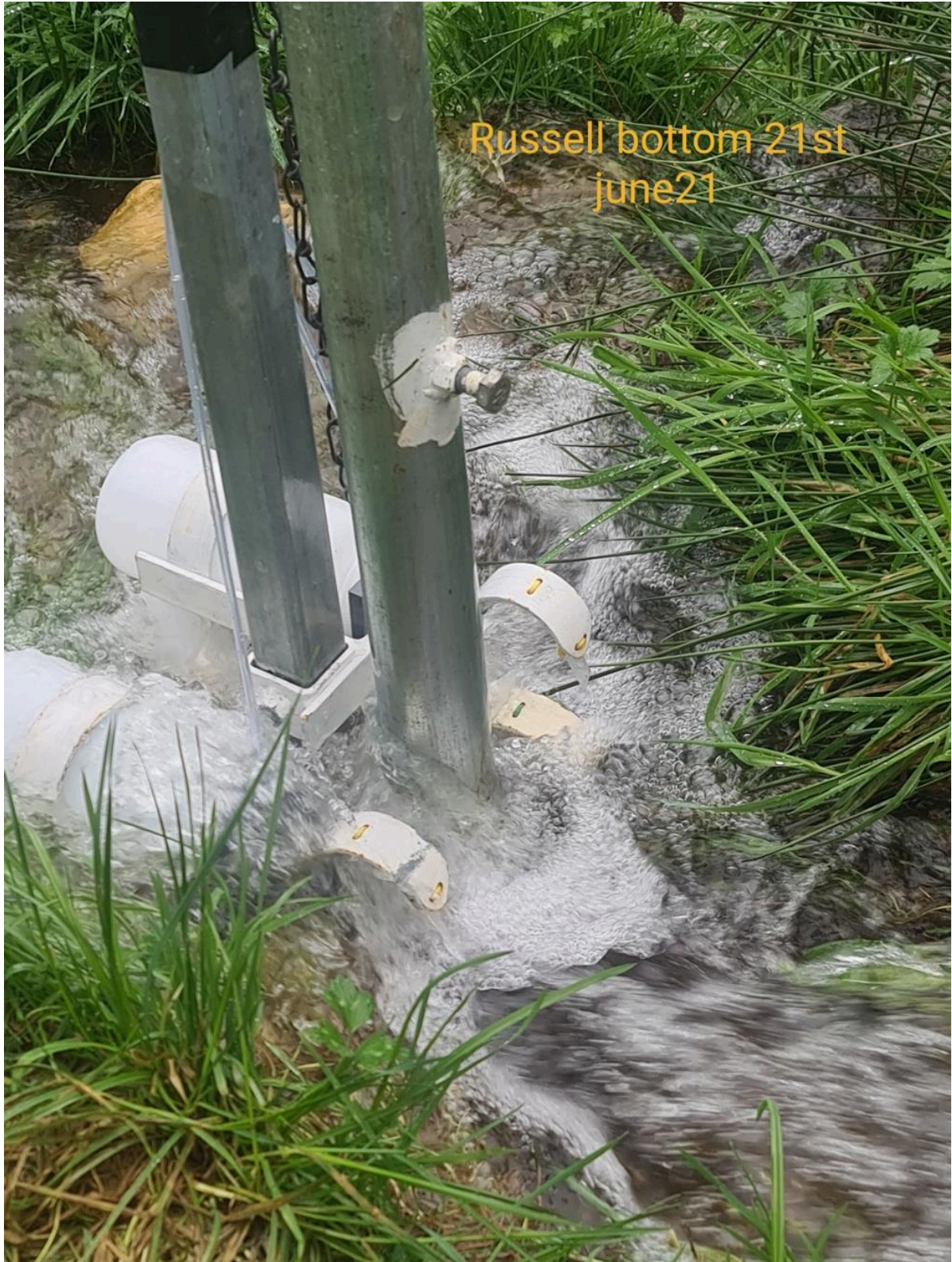
Figure 15: Water sampler working at higher inflow
