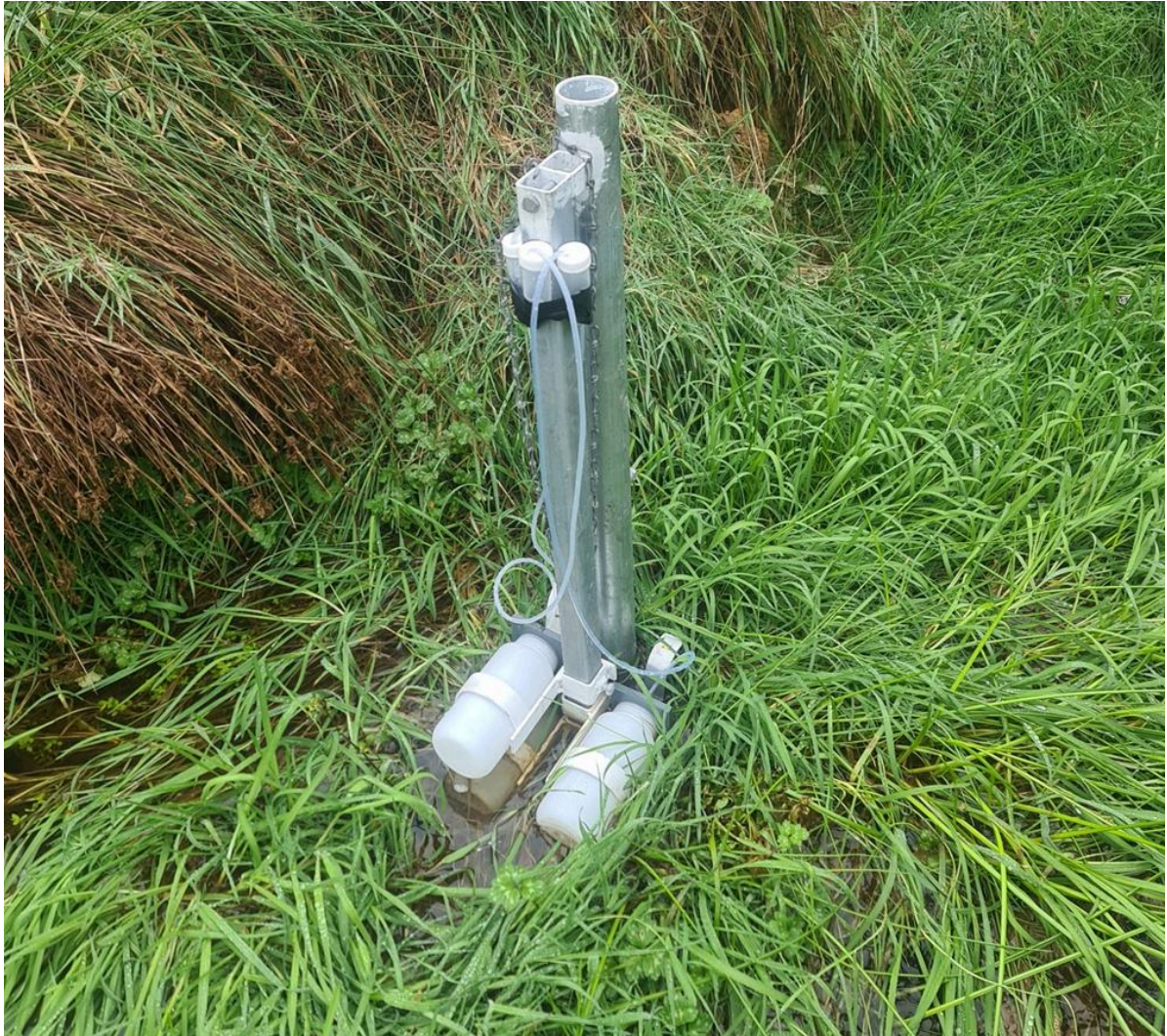
Figure 14: Water sampler set for low, medium, and high flow
