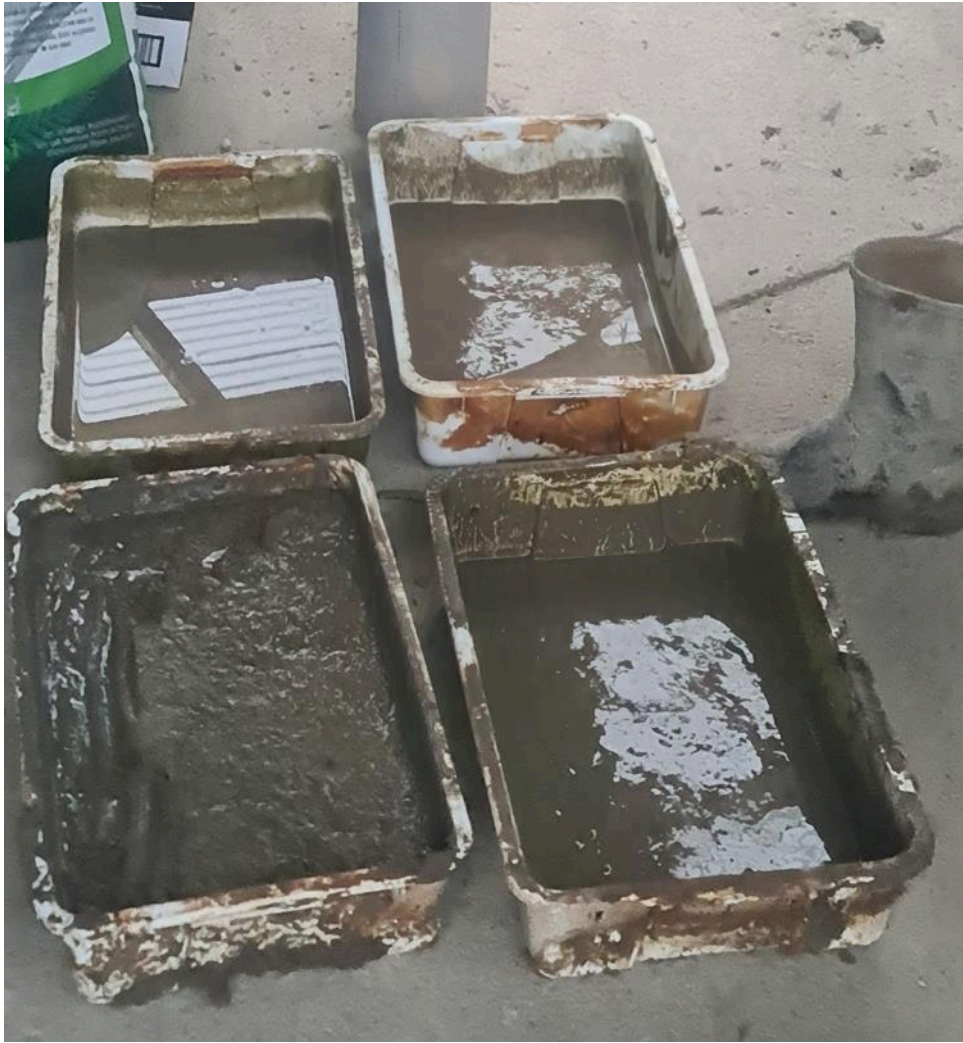
Figure 18: Sediment trays prior to drying out and weighing the remaining sediment
