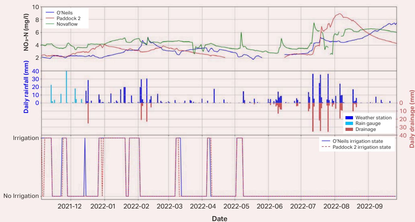
Figure 1: Extract from Appendix 3 – Nitrate results from the 3 sites (mg/L), daily rainfall (mm) and irrigation events (on/off)
