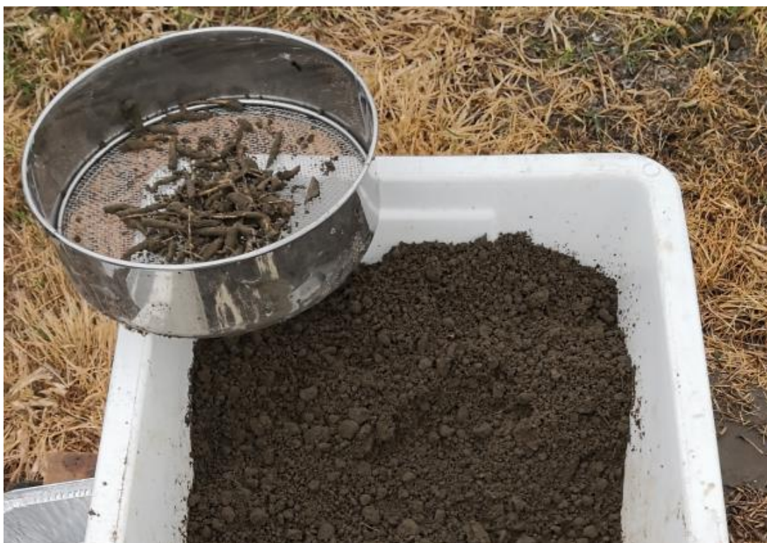
Figure 9 Roots were sifted from the soil samples using a 5 mm sieve, and sent to laboratory for washing and analysis
