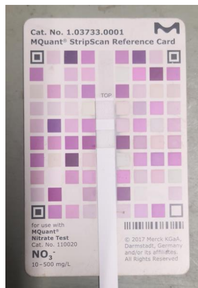
Figure 8 Test strip set on Reference Card allowing nitrate concentration to be determined using a smartphone application
